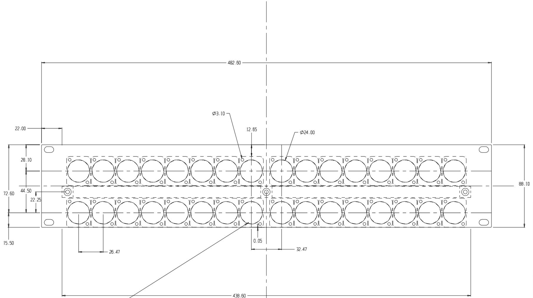
32 x NC3XLR connectors with 3.2mm fixing holes or drill 2.7mm dia and roll-form tapped M3 for MS-M3x6-CSK
