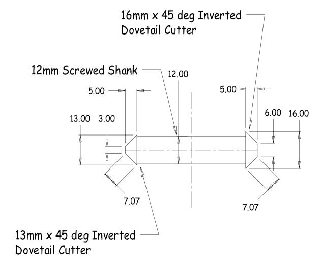
Cutting Dimension representing 2 sizes of Inverted Dovetail Cutters for bevelling CASA's Alloy plate edges & handle recesses.
