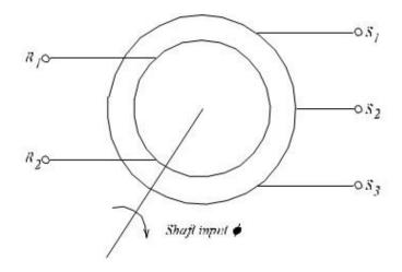
Figure - 4b Schematic Symbol of synchro control transformer
