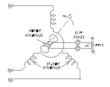
Figure - 4c Electrical Circuit of synchro control transformer
