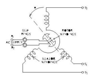
Figure - 2c Electrical Circuit (Synchro Transmitter) Where,
