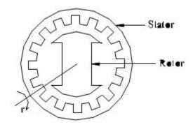
**Figure - Constructional Features of Synchro Transmitter**
