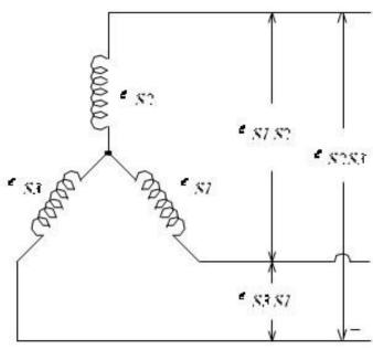
Figure -3 Induced emf in stator coils
