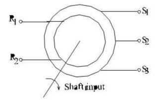
Figure - Schematic symbol of a synchro transmitter
