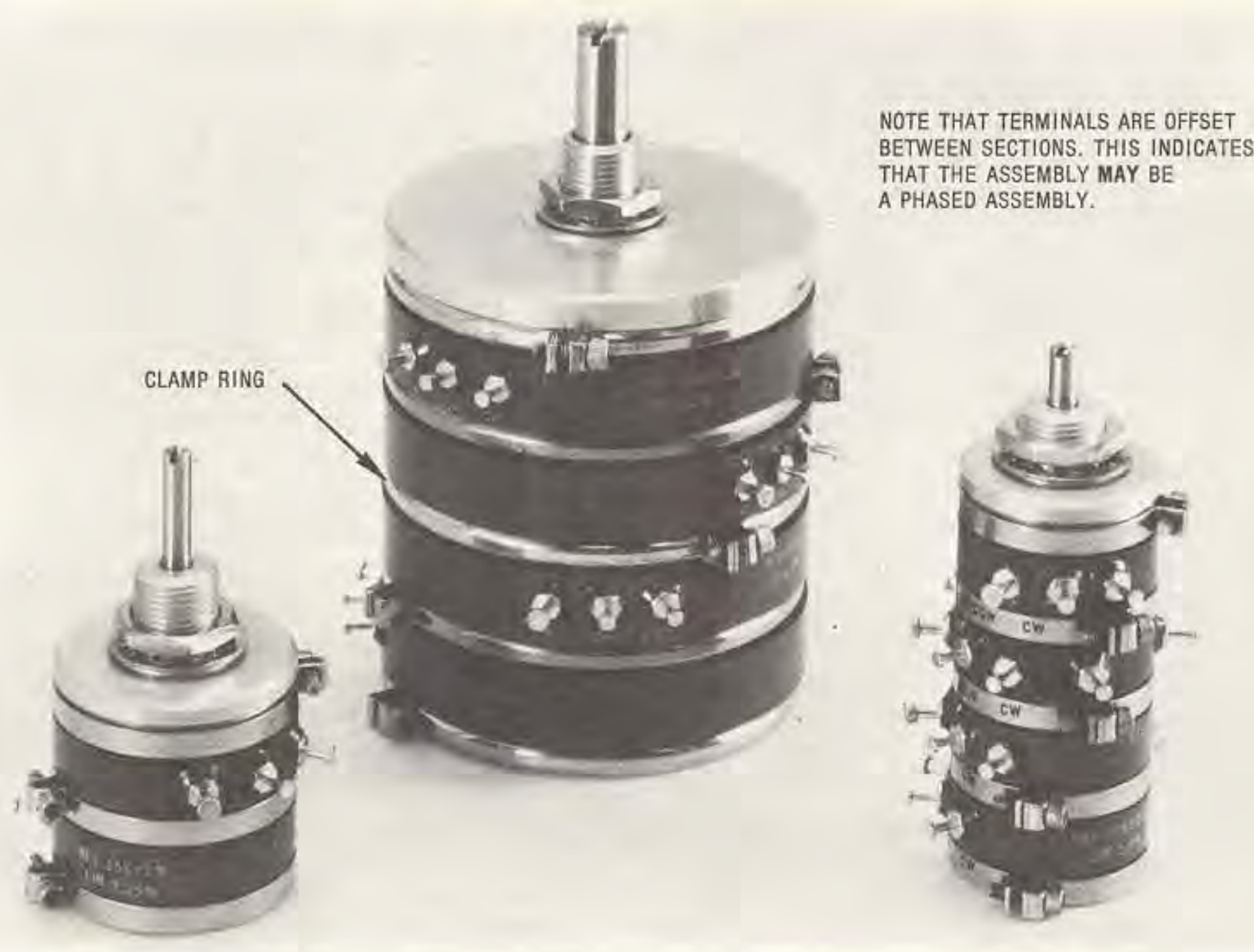
Fig. 6-16 Clamp ring style, phased potentiometer
