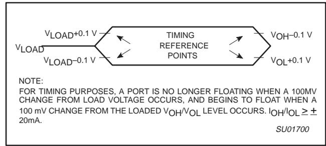
Figure 8. Float Waveform
