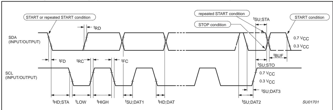
Figure 9. Timing SIO1 (I<sup>2</sup>C) Interface
