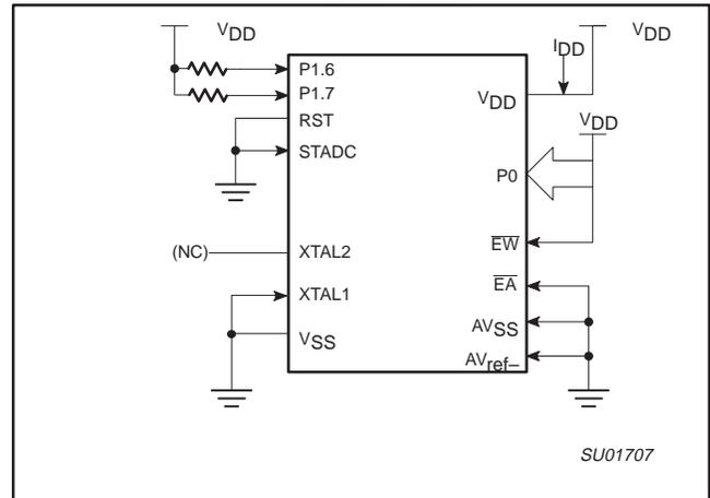
Figure 15.  $I_{DD}$  Test Condition, Power Down Mode
