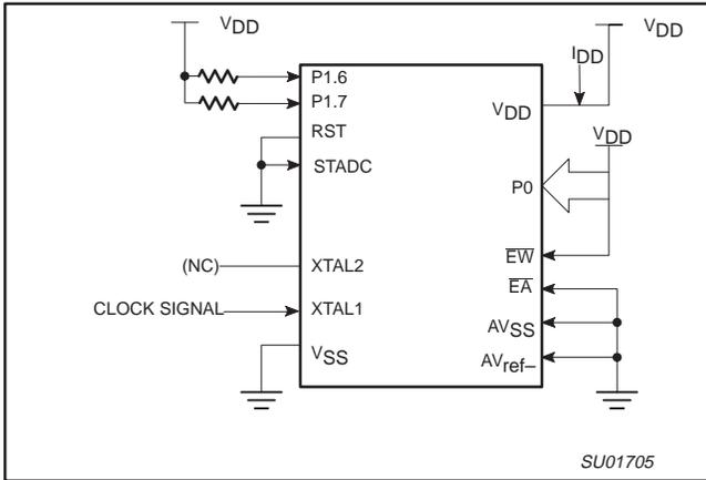
Figure 13.  $I_{DD}$  Test Condition, Idle Mode
