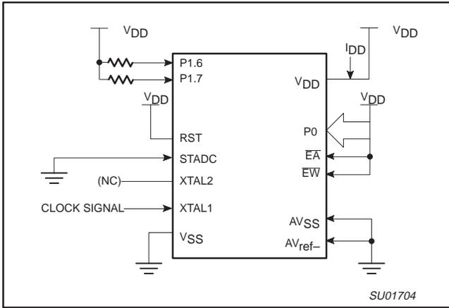
Figure 12.  $I_{DD}$  Test Condition, Active Mode
