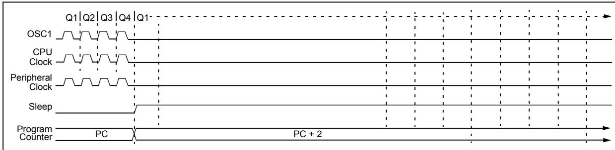
**FIGURE 4-5: TRANSITION TIMING FOR WAKE FROM SLEEP**
