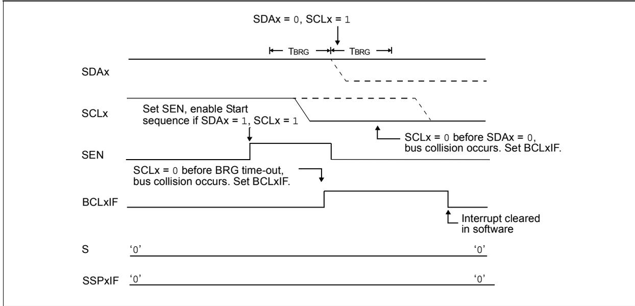
**FIGURE 16-28: BRG RESET DUE TO SDAx ARBITRATION DURING START CONDITION**
