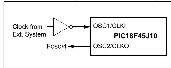
An external clock source may also be connected to the OSC1 pin in the HS mode, as shown in Figure 3-3. In this configuration, the divide-by-4 output on OSC2 is not available.
