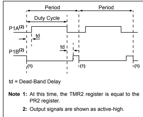
**FIGURE 15-5: EXAMPLES OF HALF-BRIDGE OUTPUT MODE APPLICATIONS**
