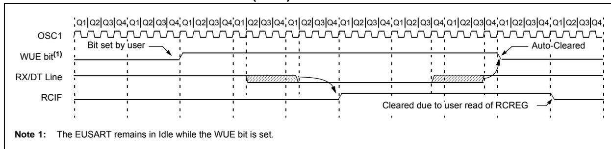
**FIGURE 17-9: AUTO-WAKE-UP BIT (WUE) TIMINGS DURING SLEEP**
