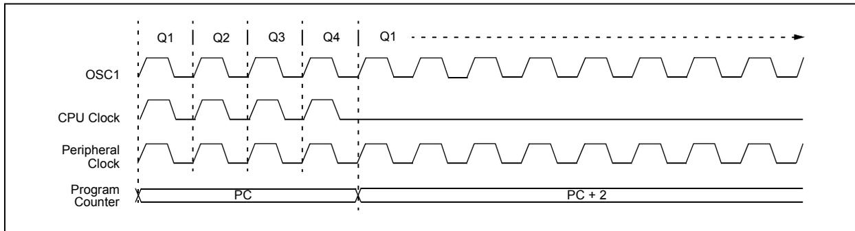
**FIGURE 4-7: TRANSITION TIMING FOR WAKE FROM IDLE TO RUN MODE**
