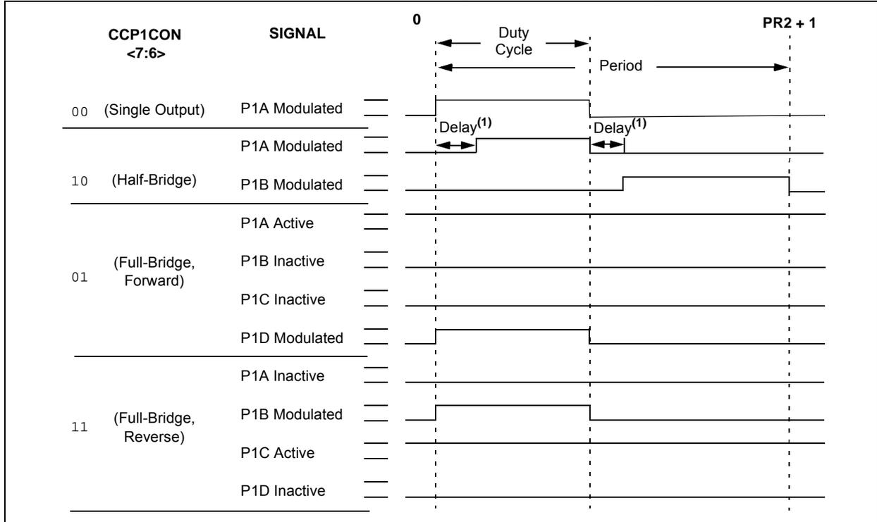
**FIGURE 15-3: PWM OUTPUT RELATIONSHIPS (ACTIVE-LOW STATE)**
