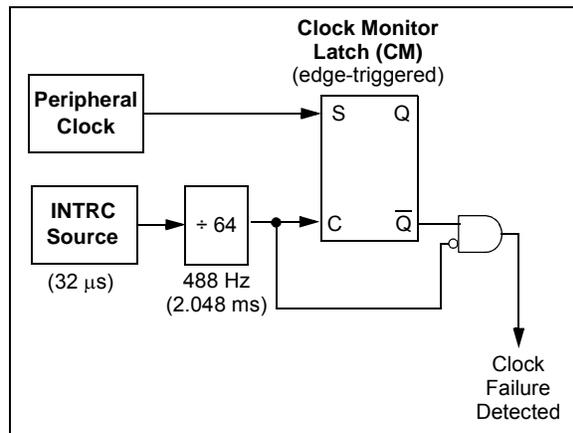
Clock failure is tested for on the falling edge of the sample clock. If a sample clock falling edge occurs while CM is still set, a clock failure has been detected (Figure 21-5). This causes the following:
