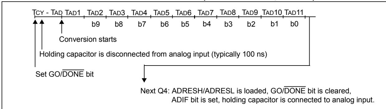
**FIGURE 18-4: A/D CONVERSION TAD CYCLES ( $\text{ACQT}<2:0> = 010, \text{TACQ} = 4 \text{TAD}$ )**
