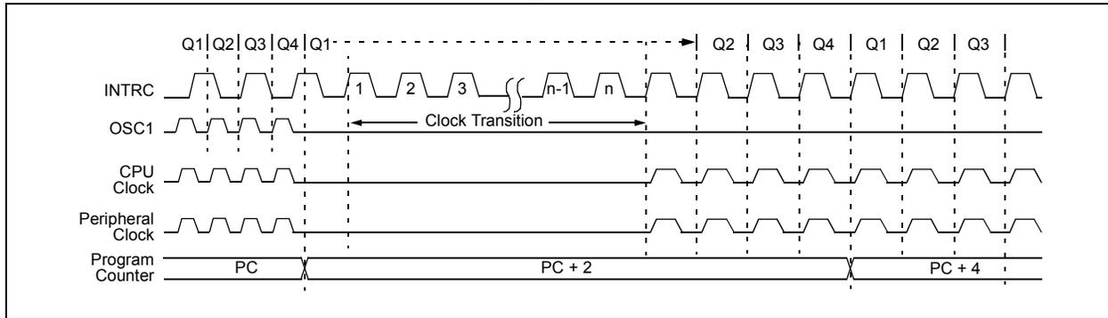
**FIGURE 4-3: TRANSITION TIMING FROM RC\_RUN MODE TO PRI\_RUN MODE**
