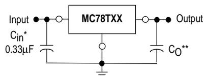
A common ground is required between the input and the output voltages. The input voltage must remain typically 2.2 V above the output voltage even during the low point on the input ripple voltage.
