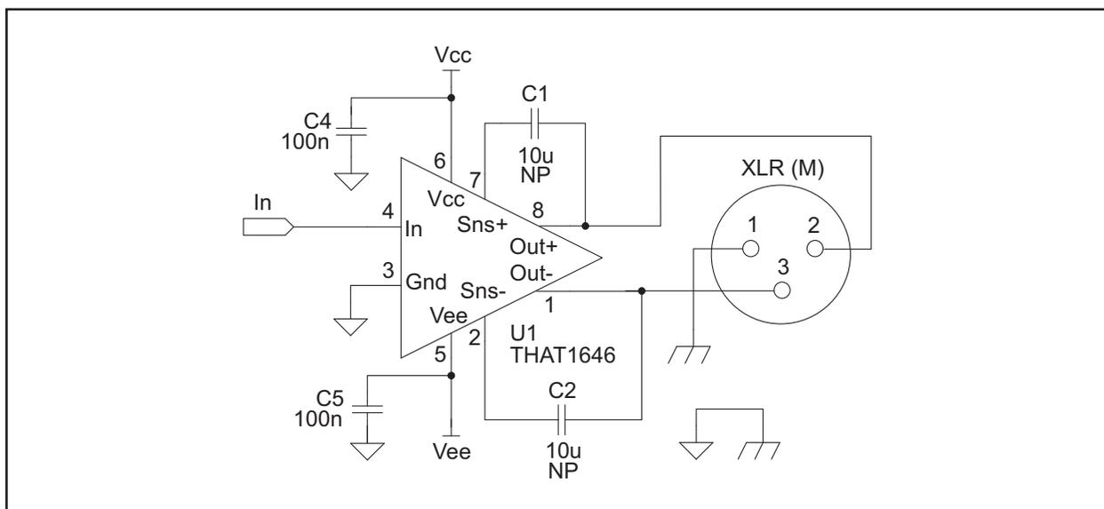
Figure 5. THAT 1646 application circuit with common-mode offset reduction
