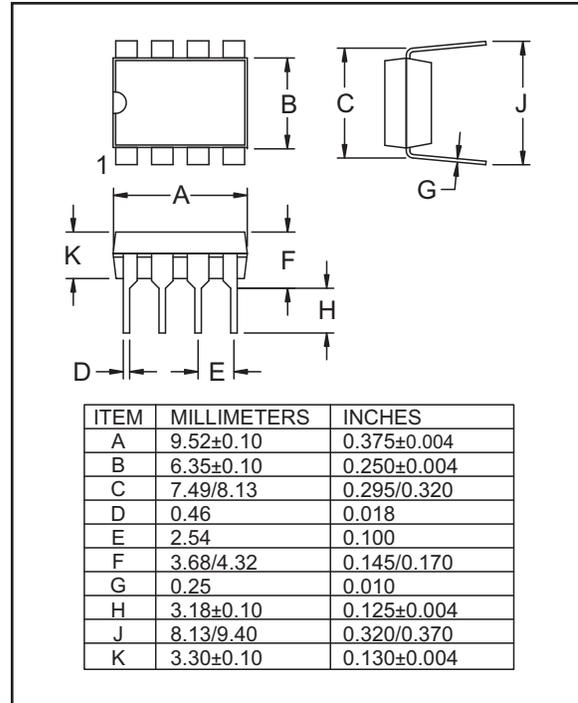
Figure 11. 8 pin DIP package outline drawing
