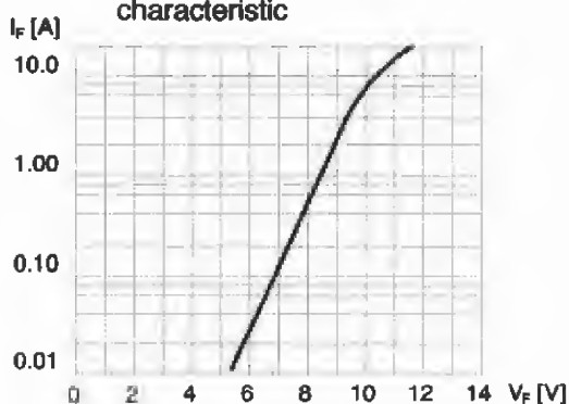
Fig. 1 - Typical forward characteristic
