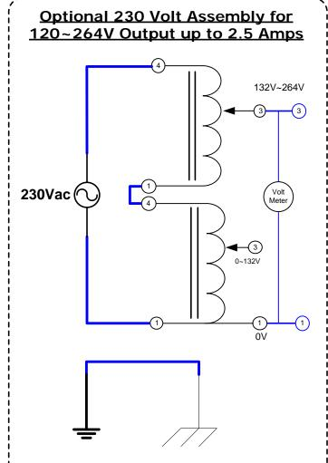
**Note:** suitable fuses or circuit-breakers must be applied to the above basic circuit.
