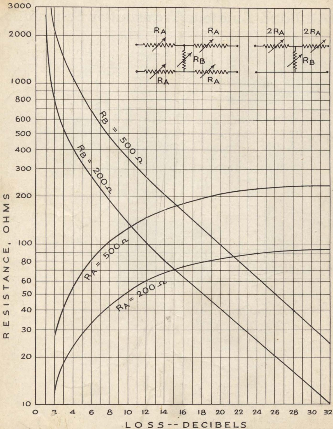
Proper attenuation of audio frequencies without introducing distortion is usually accomplished with pads. The Ken-O-Graf shown above gives resistance value of the branches of an "H" or "T" pad for channels having an impedance of 200 or 500 ohms. The range of attenuation is from 2 to 32 db.
