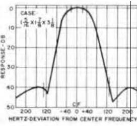
Miniaturized receiving filters, available from 425 Hz to 3315 Hz. Within 3 db at  $\pm 42.5$  Hz and attenuation of at least 36 db at  $\pm 130$  Hz. Source and load 600 ohms. Wt. approx.  $\frac{3}{4}$  lbs.
