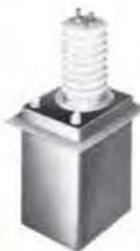
Output to Klystron. 3.5  $\mu$ sec. pulses in group of pulse trains at high rep. rate. 1% droop over pulse train. 43 KV Hipot. MIL-T-27C; NA case; 4 $\frac{1}{4}$  x 5 x 6 $\frac{3}{4}$ , 11 $\frac{1}{2}$  lb.
