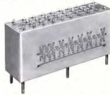
Lumped constant delay line. 15 kHz. Impedance 600 ohms. Balanced outputs tapped for delays from 27 microseconds to 118 microseconds. Delay tolerance  $\pm 1\%$ . MIL-F-18327C.
