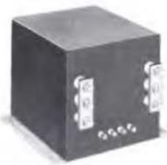
High current filament transformer. Primary 140/156 V., 47/63 Hz to 1.8 V.-1070 A. Current limiting through separate primary reactor, MIL-T-27C; 10 x 10 x 11½". 150 lbs.
