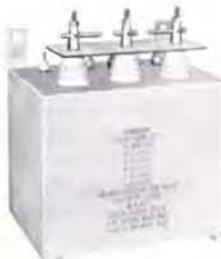
Sonar Output Transformer. 36 KW pulses, 100 millisecond @ 5% duty cycle. Input 4K  $\Omega$  CT, output 120-180  $\Omega$ . Hipot 29 KV. Hermetic, MIL-T-27C Grade 4, 6 $\frac{1}{2}$  x 9 x 8", 37 lbs.
