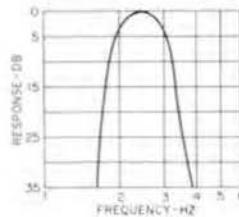
Low frequency band pass filter. From 2 to 3 Hz within 3 db. At 1.5 Hz and lower, and 4 Hz and higher, greater than 30 db. Source and load 10K ohms. MIL-F-18327C. Wt. 12 $\frac{1}{4}$  lbs. MA case, 4 x 4 $\frac{1}{16}$  x 6".
