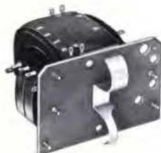
Scope power transformer with board for rectifiers. Primary 115 V., 400 Hz to two 14 KV filament windings, one 6.3 V. low capacity filament winding, 4.5 KV and 1.75 KV high voltage windings. 25 KV hipot when in oil; 2¾ x 3½ x 2¾", 1¼ lbs.
