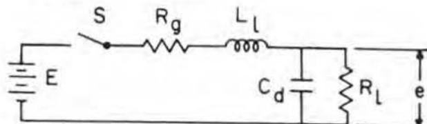
This circuit was obtained from the generalized transformer equivalent circuit by eliminating all components that are not effective at high frequency.
