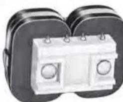
Molded High Temperature, High Voltage Transformer. Input 115 V 400 Hz, output 3400 V, 80 ma DC. Corona free molded terminals. MIL-T-27C Grade 5, Class T (170°C), 3¾ x 2¾ x 2¾", 2 lbs. 10 oz.
