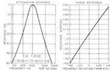
Band pass 400 Hz Gaussian filter. Linear phase response in pass band. Attenuation 380 Hz to 420 Hz within 0.5 db. 2nd harmonic down 25 db, 3rd harmonic down 45 db. Source and load 5K ohms. MIL-F-18327C. Wt., 0.9 lbs.
