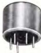
Molded carrier frequency transformer, + 8 dbm level. Within 3 db from 100 Hz to 100 kHz. 4000:4000 ohms.  $\frac{3}{4}$  Dia. x  $\frac{5}{8}$  inches,  $\frac{1}{2}$  oz.
