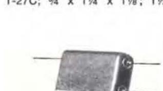
Differentiating pulse transformer. Input 150 V. 40 MA peak, 6  $\mu$ sec., 3000 PPS. Output 30 V. .5  $\mu$ sec. Ferrite core. Rise, droop, and pulse duration held to 5%. MIL-T-21038B, -55° C. to + 100° C.; 5/16 x 5/8 x 1; 7 grams.
