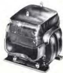
Linear charging reactor for line type pulser. 20 Hys., .11A. DC, 5 KV, 1000 PPS, 11 KV hipot. MIL-T-27C, 200° C.; 3 $\frac{1}{4}$  x 4 x 3 $\frac{3}{4}$ , 3 lb.
