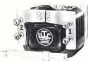
Impulse Transformer, discharge 37.5 mfd. Capacitor @ 5 KV DC, Peak Current 167,000 amps. Pulse width 2  $\mu$ sec, Rise time .2  $\mu$ sec, Energy level 470 watt-sec. MIL-T-27C Grade 5, Size 10 x 12 x 9 $\frac{1}{2}$ ", 135 lbs.
