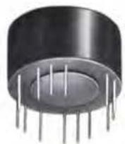
Self-saturating inverter transformer; 100 V DC input. Frequency of oscillation 20 kHz. MIL-T-27C, Class T. Size: 1.25 Dia x .60 H, PC mounting.
