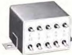
Thirty Hz cathode follower output transformer to provide equal voltages to 4 loads and supply a half-wave rectifier. Primary inductance maintained to 5% with 20% change in DC unbalance and 30% change in AC voltages.
