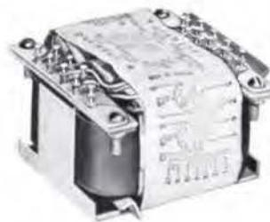
230° C. power transformer. Primary 115 V., 3 phase, 300/420 Hz to 200 V. and 20 V. secondaries, 525 V.A. 230° C. operating; 2¾ x 3 x 2", 1.8 lbs.
