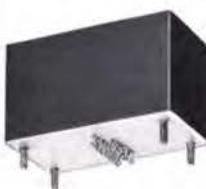
Precision Magnetic Modulator and Filter to produce sine wave output directly proportional to a DC control input. Temperature stabilized from -55°C to 85°C. Distortion and linearity less than 3% thru temperature and frequency range of 380-420 Hz. MIL-T-27C, 1¾ x 1¾ x 3⅛", 12 oz.
