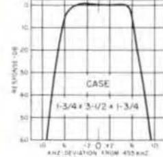
Crystal filter, 455 kHz. Source 70 ohms, load 5K ohms, 6 db bandwidth, 11 kHz minimum. Shape factor 60 db BW/6 db BW = 1.75/1. Max. ripple 1 db, Wt. 0.5 lbs.
