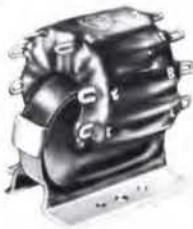
High temperature power transformer. Primary 115 V., 320/1000 Hz to four 6.3 V. and one 475 V. secondaries, 200° C. MIL-T-27C; 2¼ x 2 x 2", 9 ounce.
