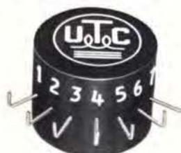
Instrument reference transformer. To operate from 15 kHz to 20 kHz with 12.5 V on one half of primary and to deliver 9.0 V on each half of secondary; secondary halves loaded with different impedances. Size: 1.1 Dia. max. x .79" high max. Weight: 34 gms.
