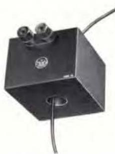
Current Transformer with 1 K load exhibits 1 V/amp/turn sensitivity. From 400 Hz to 30 kHz,  $\pm 0.1$  db. Good linearity with both current, 1 mA-10 A; and turns, 1-5 T.
