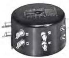
Toroidal Transistor inverter transformer. Input 24 V DC, outputs 4 windings 150 V to 1050 V DC. Hipot 3800 V. Hermetically sealed, MIL-T-27C, 2½ dia. x 1¾", 15 oz.
