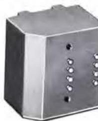
Dual saturable reactor. Input 10 V. - 1 kHz. Output 3.5 V. 2 MA DC control current. 130° C. MIL-T-27C; 1¾ x 1¾ x 1¼, 5 oz.
