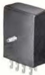
Gaussian wave shape pulse output. Input 2 KV, 3.5  $\mu$ sec. Output 2.5 KV-5A., 80 kHz rate. Corona free-35,000 feet. MIL-T-27C; 1 $\frac{1}{8}$  x 1 $\frac{1}{8}$  x 3 $\frac{3}{8}$ , 1 lb.
