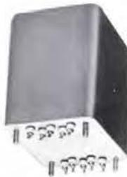
Magamp for 50 watt, 60 Hz servomotor. Two control windings. One feedback winding, one power winding, diode panel. Power gain 100. MIL-T-27C; 30 lbs.
