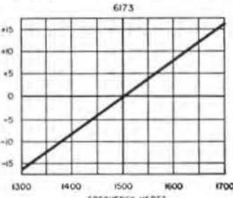
UTC high Q discriminators provide exceptional amplification and linearity. Values are volts.  $1\frac{1}{16}'' \times 1\frac{1}{16}'' \times 3''$ .
