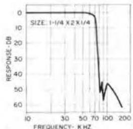
Ultra-miniature low pass filter only 1/4" high. DC to 40 kHz within  $\pm 0.1$  db, within 1 db to 60 kHz, 3 db to 70 kHz. Attenuation of at least 40 db above 81 kHz. Source and load 1K ohms. MIL-F-18327C. Wt. 1.2 ounces.
