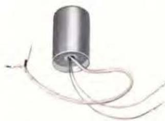
Microphone input transformer, double drawn hipermalloy shields. Shielded cable leads. Ratio 100:1.  $1\frac{1}{16}$  Dia. x  $1\frac{1}{2}$ " high. Inductance greater than 1000 Hys. at 60 Hz.
