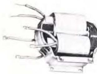
Output to magnetron. Input 6 KV peak 2.5  $\mu$ sec. or .5  $\mu$ sec. Output 28 KV-27 A. peak and 14.2A. bifilar magnetron filament winding. MIL-T-27C, 170° C.; 2 $\frac{1}{2}$  x 5 $\frac{3}{8}$  x 4 $\frac{1}{8}$ , 7 $\frac{1}{2}$  lb.
