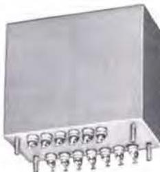
Servo reference transformer. Input 120 V., 380 to 420 Hz. Output ratios under load held to .005% tolerance. Phase shift .05° max. MIL-T-27C; 2½ x 1¾ x 2, 12 oz.
