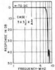
Low pass filter, 6 MHz. DC to 6 MHz within  $\pm 0.1$  db. Attenuation at least 40 db at 8.5 MHz and higher. Source and load 75 ohms. Wt. approx. 8 oz.
