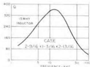
Type MQV, 15 millihenries temperature stable inductor. High Q in the 2 kHz to 50 kHz frequency range. MIL-T-27C. Wt. 14 oz.
