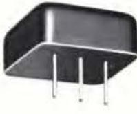
Telemetering low pass filter 560 Hz. Available from 400 Hz to 70 kHz.  $\pm 7.5\%$  bandwidth flat to 1 db. Attenuation greater than 35 db beyond the 2nd harmonic of  $-7.5\%$  frequency. Impedance 47K ohms. MIL-F-18327C. Wt. 0.8 oz.
