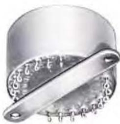
Multi Control Magamp. Power gain 400,000. Control Current .00003A. Output 25 V. DC into 1K. Six power windings, bias, feedback, and two control windings. MIL-T-27C; 2½ dia. x 1¼ high, 8 oz.
