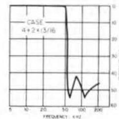
Sharp cutoff 49 kHz low pass filter. Stable to .1 db in pass band from 0°C. to 85°C. Within 1 db 5 kHz to 49 kHz, over 40 db at 56 kHz. MIL-F-18327C; .6 lbs.
