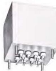
High voltage, constant inductance, tapped inductor. 16 millihenries, 8 kHz, inductance variation less than 1% from 1 volt to 1600 volts. Q greater than 40 at 1600 volts. Case size: 3 1/16 x 3 1/16 x 2 1/4" high. Grade 4, MIL-T-27C.
