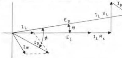
The diagram shows the result of the transformer parameters considered in the equivalent circuit and their terminology.
