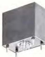
Bolometer transformer. Primary 10 ohms, secondary 530K ohms, 230:1 ratio, response from  $\frac{1}{2}$  Hz to 25 Hz. 120 db magnetic shielding, to 25 Hz. 120 db magnetic shield-plus full electrostatic shielding.
