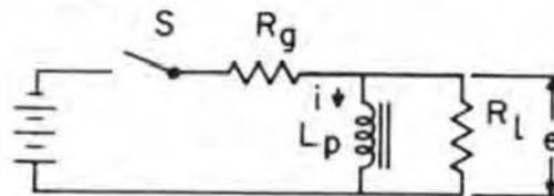
This circuit was obtained from the generalized circuit by eliminating all components that are not effective at low frequency.
