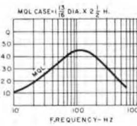
Since these high Q coils will saturate before any appreciable temperature rises occur, heating is usually not a problem. A general rule would be that 4 times the DC listings may be applied without any detrimental heating due to copper loss.
