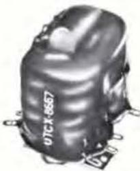
Output to 2J42 magnetron. Input 1300 V-.50 ohms. Output 6.5 KV to 1200 ohms and .6A. bifilar filament winding. .15  $\mu$ sec., 1000 PPS. Trigger winding. MIL-T-27C Grade 5; 1 $\frac{1}{2}$  x 2 $\frac{1}{2}$  x 2 $\frac{3}{4}$ , 10 oz.
