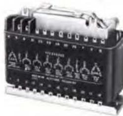
Molded Power Transformer 3 Phase. Input 200V, 380-420 Hz Electrostatic Shield, 8 output windings. 26 terminals. MIL-T-27C, Grade 2 Class S. Max. Alt. 50K Ft. Size 6 x 2½ x 5", 8 lbs.
