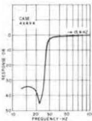
High pass filter, 30 Hz, used to eliminate from the output, 25 Hz sine wave pulses which control automatic programming on audio tracks of music tapes. Flat to 1 db from 50 Hz to 15 kHz, within 3 db to 30 Hz. Attenuation of at least 35 db from 25 Hz to 20 Hz. Source and load 600 ohms. Wt. approx. 6 lbs. MIL-F-18327C.
