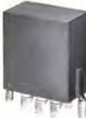
Free running blocking oscillator transformer. 600 ohms, 1:1:1, 5  $\mu$ sec. ± 1, 12000 ± 10% PPS. Output 600 V. ±10%. Temperature stable -62° C. to 85° C. MIL-T-27C; 3 $\frac{1}{4}$  x 1 $\frac{1}{4}$  x 1 $\frac{1}{8}$ ; 1 $\frac{1}{2}$  oz.
