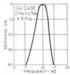
Twelve Hz band pass filter. From 11 thru 13 Hz attenuation less than 2 db. At 7 Hz and at 17 Hz, attenuation greater than 40 db. Source and load 50K ohms. MIL-F-18327C. Wt. 2.5 lbs.
