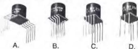
BIT-P's stock units are manufactured with Flat Pack type terminations extending outward. Terminations may be bent for adaptation to plug-in applications. Unique termination configuration isolates strain and affords safety during bending process. Variations of bends are pictured above.
