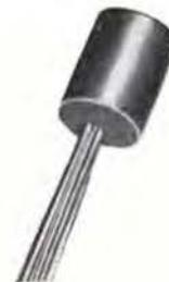
DO-T Pulse Transformer, width 150  $\mu$ sec., ratio 1:1:1. Transistor output to gating circuits. -65°C to 105°C. MIL-T-21038B. 5/16 Dia. x 13/32, 1/10 oz.
