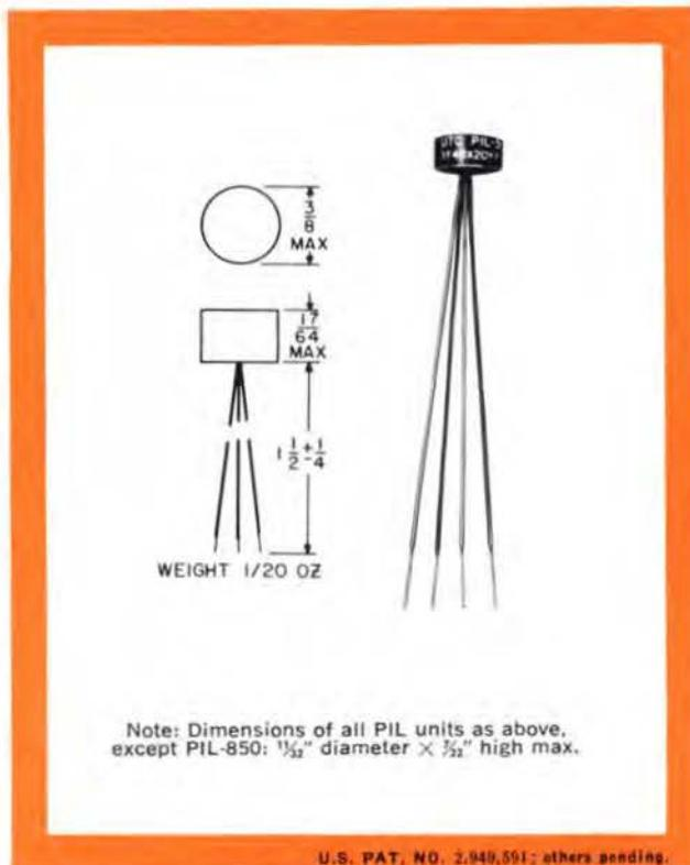
Note: Dimensions of all PIL units as above, except PIL-850:  $1\frac{1}{32}$ " diameter  $\times \frac{7}{32}$ " high max.
